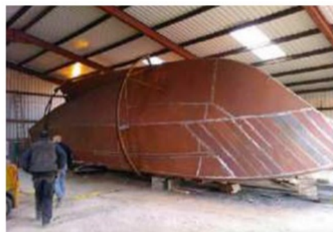
BELOW: Turning the new 55ft hull using a temporary cradle
